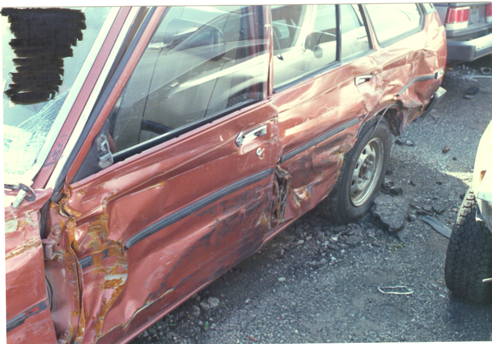
Rearward Displacement Of The Leading Edge Of The Left Front Fender and Door.
